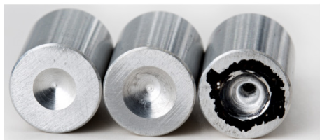
Fig. 2. Unused, pulsed sputtered and continuously sputtered cathodes (from left to right).
